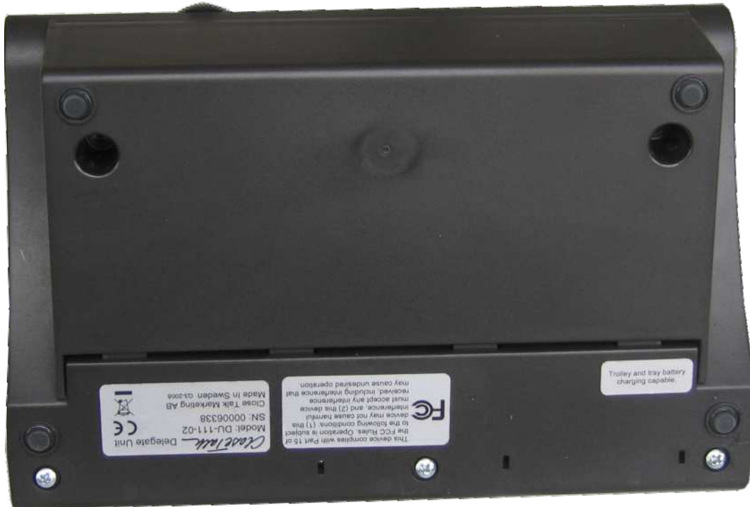
Fig. 18: Replace the battery cover, making sure it fits properly on all sides
