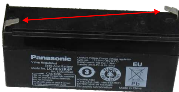
Fig. 10: The Panasonic battery type has its terminals on the opposite diagonal corners
