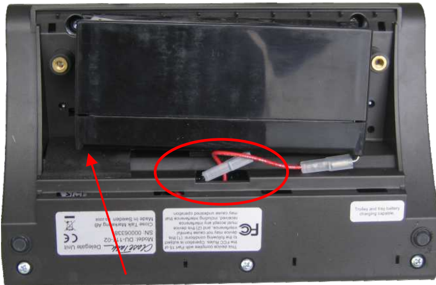
Fig. 14: The Panasonic battery with correct placement. The image shows the new soft plastic connector housing. The arrow is pointing to the correct negative pole placement
