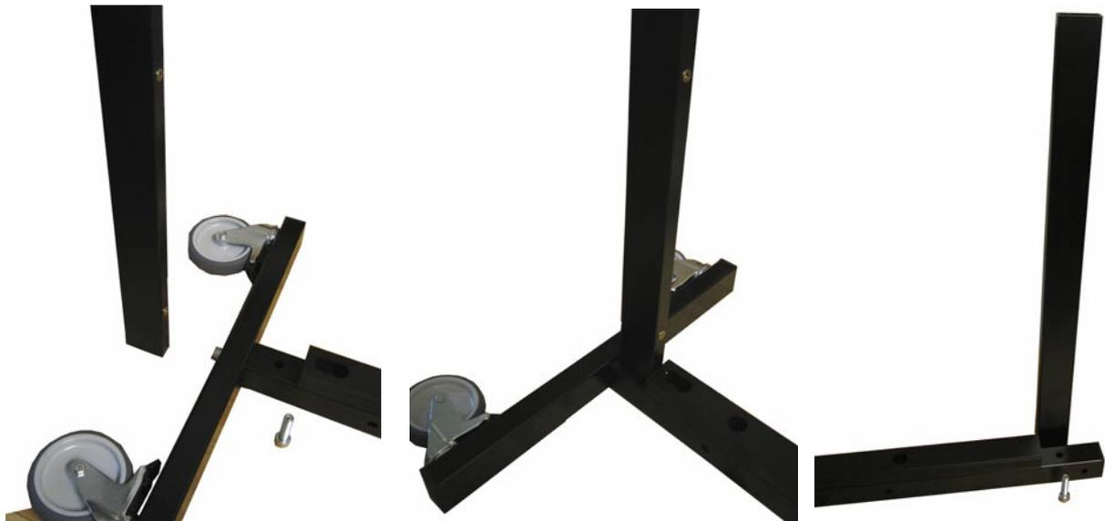
*Start with the cable conduit wheel side, be sure to mount the power supply screw holes on the lower beam next to the cable conduit lower exit holes as shown on the left and middle image. Use two 8mm size screws to securely fasten the two horizontal beams.*
