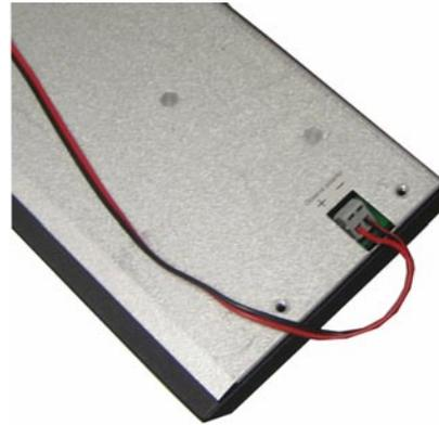
*Observe polarity or the unit will be damaged!
