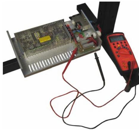
*Use DC voltmeter to verify supply voltage*
