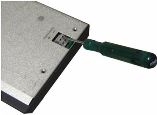
*Insert the flat nose screwdriver, carefully twist it to open the contact and insert the stripped cable end. Make sure it contacts properly and that no possible short-circuits exists*
