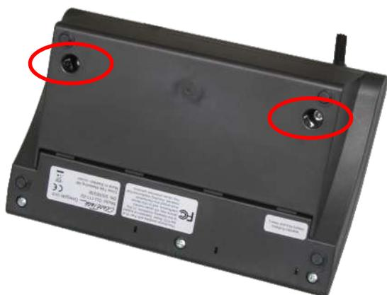
Fig. 2: Delegate unit upside down, cover holding screws are circled
