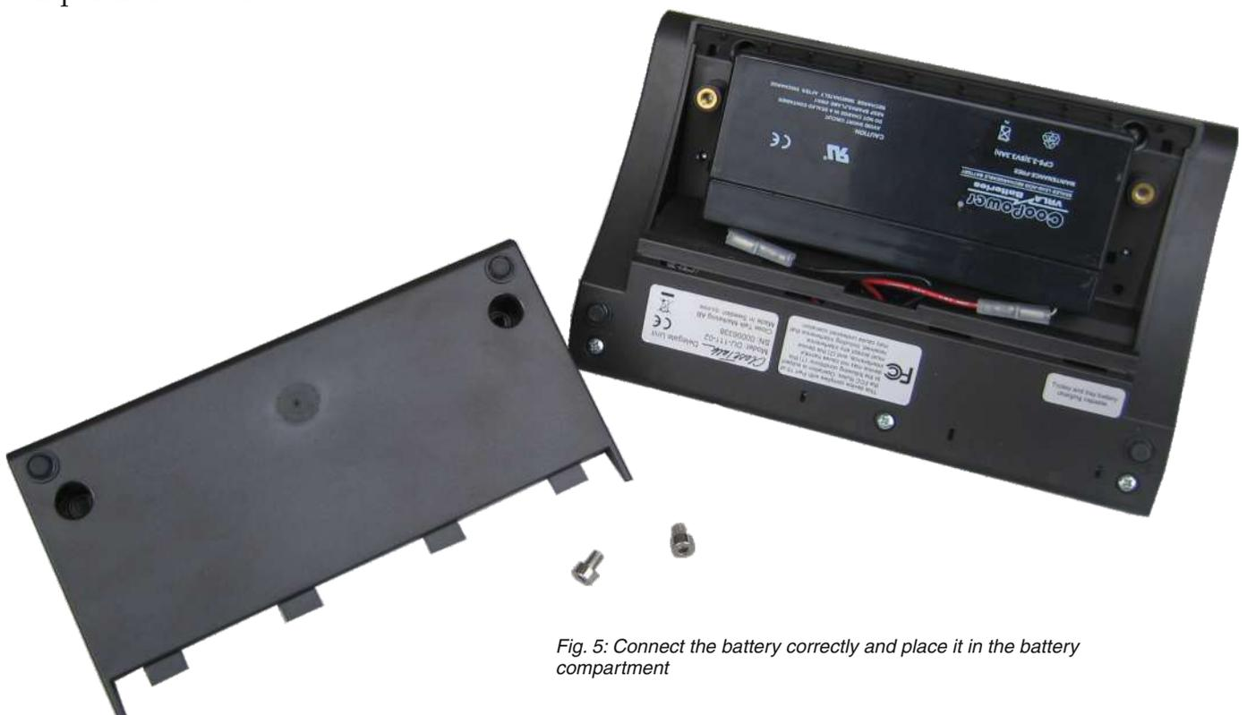
Fig. 5: Connect the battery correctly and place it in the battery compartment
