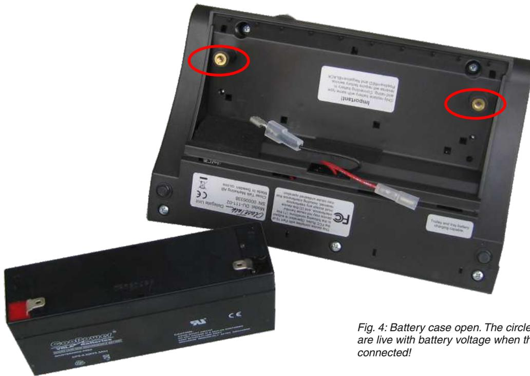
Fig. 4: Battery case open. The circled brass threads are live with battery voltage when the battery is connected!
